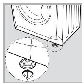
If the tumble dryer is not perfectly level, use a wooden block to support it while you adjust the two front feet, making them taller or shorter as necessary.
