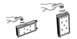
Whilst the condenser is removed, clean as much fluff as possible from inside the ducting by reaching a hand into the machine. In particular, keep the passage from the fan clear (on the right hand side of the condenser duct).
