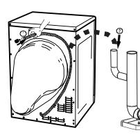
To return your drier back to taking the condensed water to the water bottle, simply fit the drain hose back to the valve at the top of your drier.
