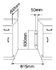
The illustration shows the minimum space required by the dryer and the position of the waste-pipe within this space and behind the dryer. If a trap is fitted it must not obstruct the air inlet at the back of the dryer. The waste pipe can be positioned on either side of the dryer. If the waste pipe is used by the dryer and a washing machine then its diameter must be large enough to contain both hoses - 1.5" bore (38mm)
