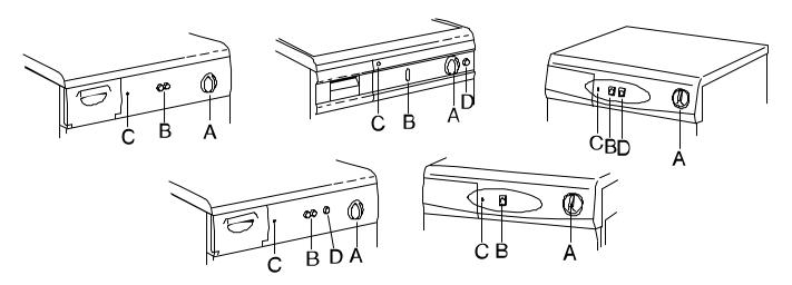
A. THE TIMER Select the required drying time based on the recommendations on the control panel.B. HEAT SWITCH(ES) Select the required heat setting based on the recommendations on the
