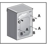
**Step 3**. Remove the 3 retaining screws (A) at the rear of the machine, as indicated in the image on the left.
